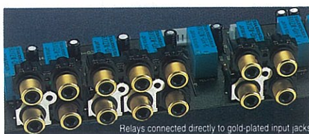
Relays connected directly to gold-plated input jacks
